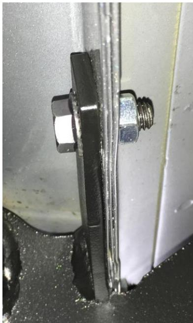
**Step 7:** Next, adjust the step assembly up/down and front/back to level out the step rail with body panel and then tighten step to brackets at 30 ft. /lbs.
