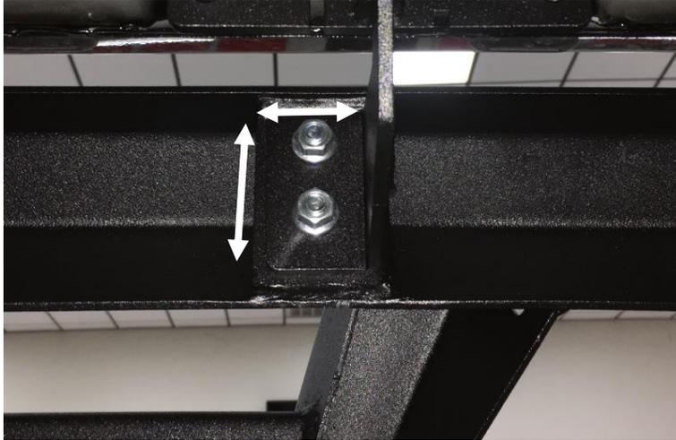
**Step. 8:** After final positioning, completely tighten all (x6)  $\frac{1}{4}$ "-20 x  $\frac{3}{4}$ " in the pinch weld attachment.
