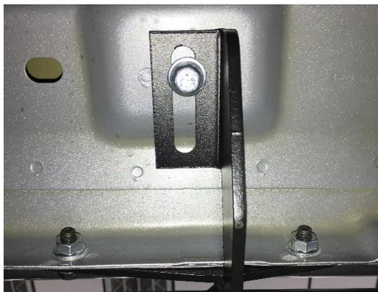
**Step. 6** Next, start all (x6) 1/4"-20"x 3/4" hex bolts, (x12) M8 flat washers, (x6) 5/16" lock washers and (6) 1/4"-20 HC Nut in the pinch weld mounting locations and leave loose for now.
