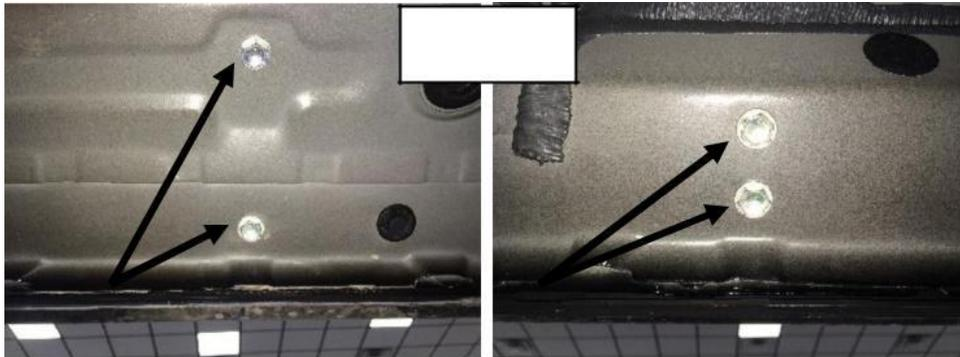
**Step 4:** Position step assembly up to the body of the vehicle and align the brackets up with the factory mounting locations.
