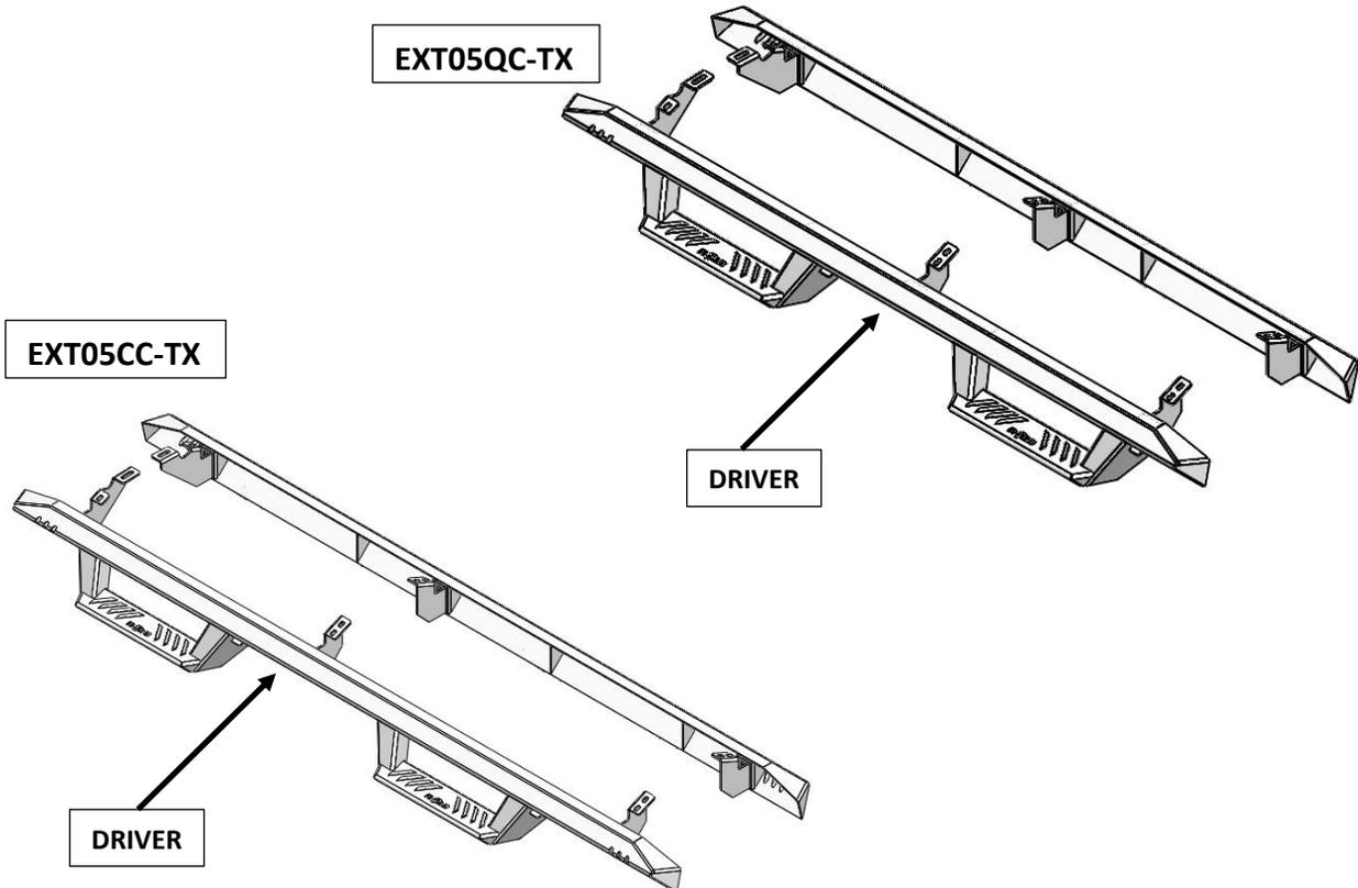
**Step 2:** Install three rocker panel brackets to the attachment points located on the backside of the channel using the supplied 3/8" x 3/4" carriage bolts and 3/8" flanged nuts. Leave finger tight for now.
