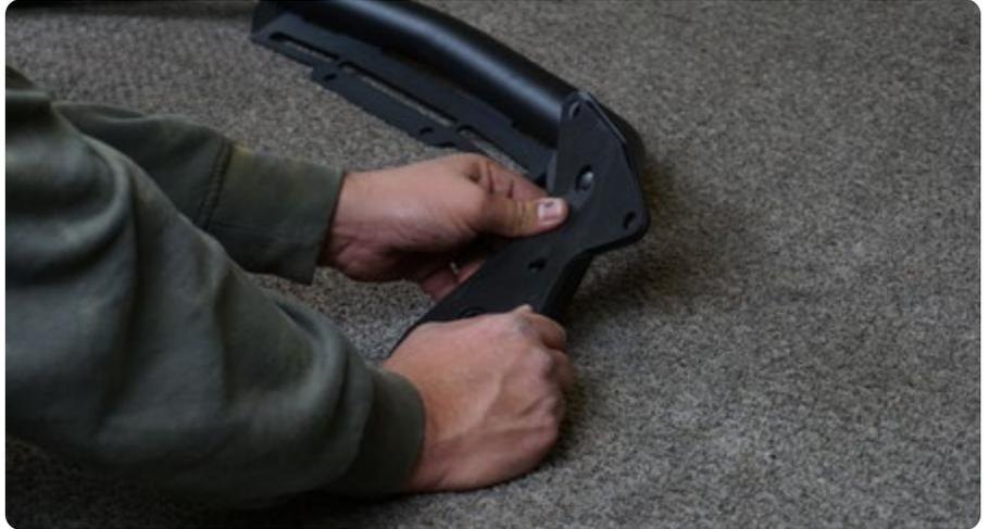
**STEP 7** | Loosely install bull bar onto the bumper using the provided M8x25 allen head hardware.
