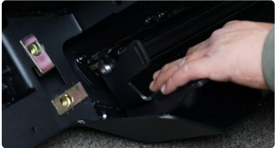
Install the bumper support braces using the provided M12x30 hex hardware with a 18mm and 19mm socket or wrenches.
