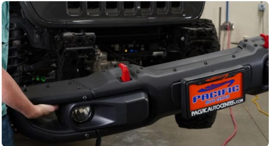
**STEP 5** | At this point, frame rails should be visible and the vehicle should be ready for installation of an aftermarket bumper.
