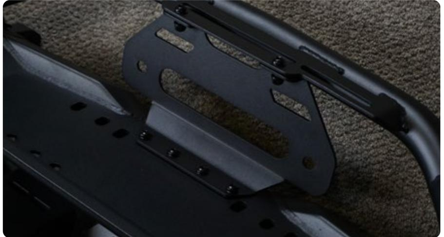
**STEP 9 |** Install flat nuts on the bumper by sliding them into place. These can sometimes require a little force to install.
