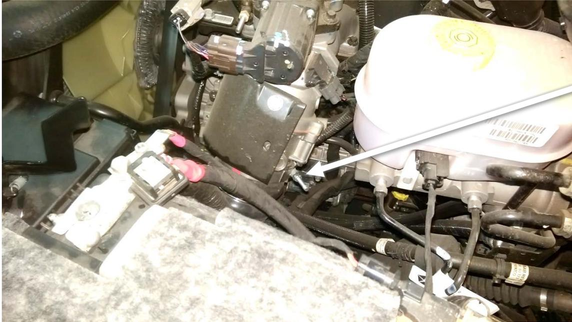
Figure 5c (DRIVER SIDE INTERCOOLER CLAMP)
