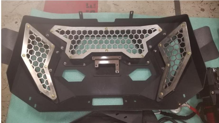
3. If installing an Adaptive cruise control module install module to the included bracket using the provide M8 nuts. Then install bracket to grill section using the 2 lower center insert 5/16" bolts
