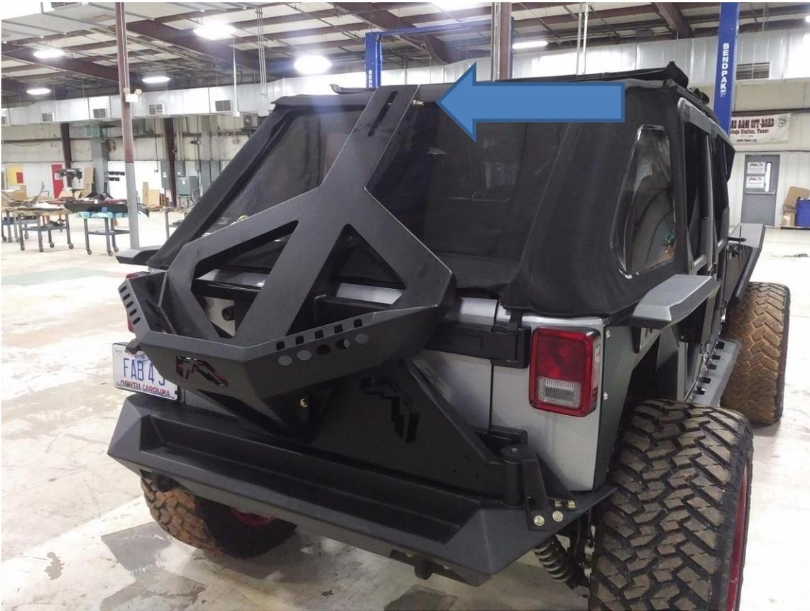
3. Using the provided 3 point tire strap tighten tire to tire carrier.
