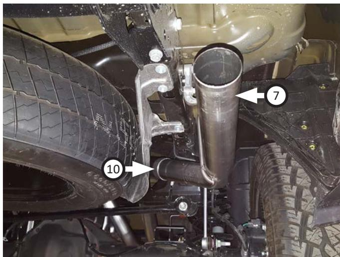
16. Place (x2) **tips (8)** onto exit pipes and tighten inlets. Rotate exit pipes and tips to desired distance from body or bumper, so angle cut on tips are properly positioned.
