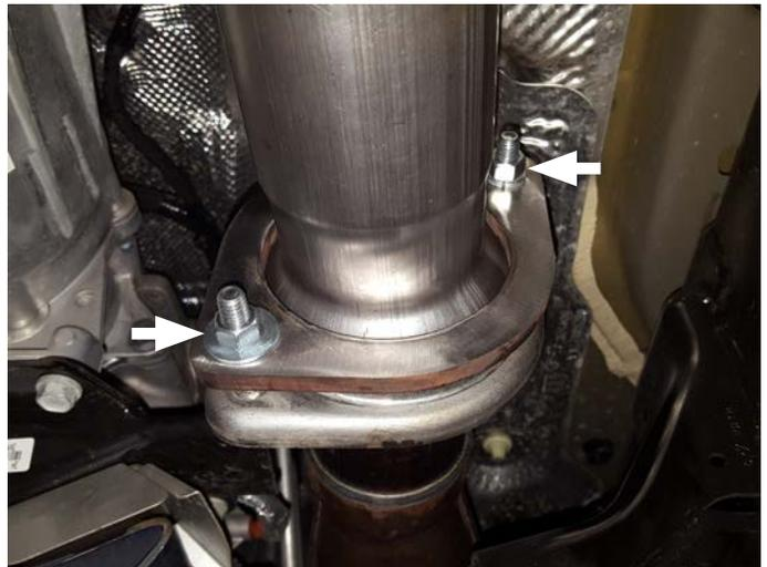
11. Place **clamp (9)** onto **extension pipe (2)** then connect them to inlet pipe. Insert wire hanger into isolater and plug in grounding wire (removed step 5). Tighten clamp just enough to allow for adjustment.
