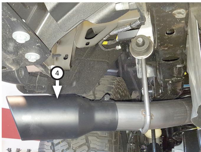
11. Adjust exhaust components for fit; maintaining ½" clearance and compensating for suspension, travel and vibration then tighten all clamps.
