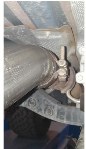
7. Place **clamp (3)** onto **muffler (2)** then connect it to inlet pipe. Tighten clamp just enough to allow for adjustment.
