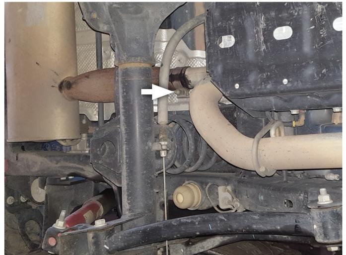
4. Loosen ball clamp from resonator inlet, disassemble hanger wires from isolators and remove resonator section from vehicle. Release tab to remove clamp from pipe and retain it for later use.
