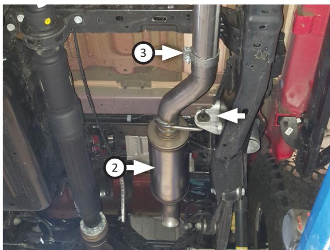
8. Adjust exhaust components for fit; maintaining  $\frac{1}{2}$ " clearance and compensating for suspension, travel and vibration, then tighten all clamps.
