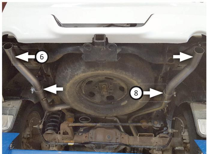
13. Place **stainless tips (7)** onto both exit pipes and adjust to desired position. Tighten pinch clamps enough to hold in place.
