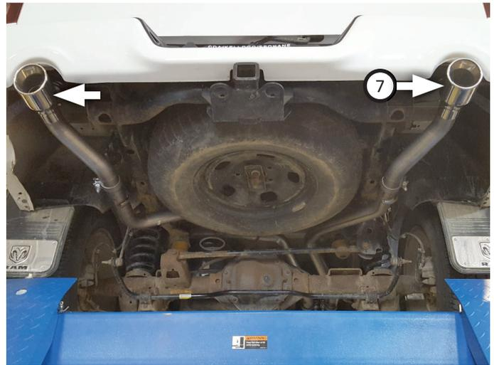
14. Adjust exhaust components to provide a satisfactory fit. Maintain a minimum of  $\frac{1}{2}$ " clearance around all components of exhaust system, keeping in mind suspension, travel and vibration. After making any required adjustments, securely tighten all clamps.
