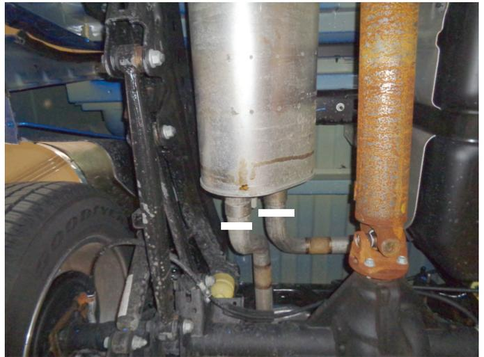
4. Support muffler with a stand, remove muffler wire hangers from isolators then loosen ring clamp at muffler inlet connection. Slide muffler off of front pipe and set aside.
