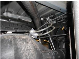
6) Place left front tailpipe section **#26430S** into position over the rear axle and slide into the left muffler outlet. Place a supplied 3" clamp onto the back of the pipe. Place left rear tailpipe section **#26432S** onto the front section, and connect the hanger welded to the rear of the pipe into the rubber hanger installed in step 3 above. Pipe should be centered between the shock and the spare tire when adjusted. Tighten the clamps just enough to hold in position.
