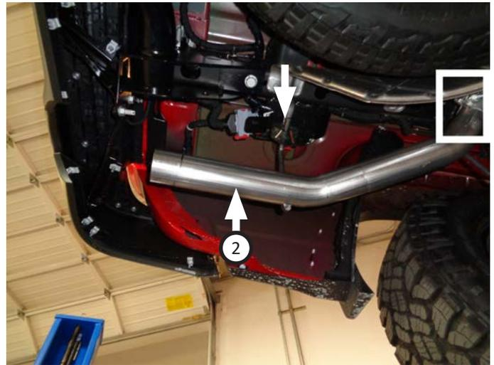
7. Place **clamp (4)** onto **right tailpipe (1)**. Connect left tailpipe to left exhaust outlet and insert wire hanger into isolator. Tighten clamp just enough to allow for adjustment.
