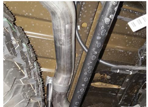
12. Place **clamp (8)** and rear hanger mount (removed step 3) onto **left exit pipe (5)** then connect it to y-pipe left outlet. Re-install rear hanger mount then tighten clamp just enough to allow for later adjustment.
