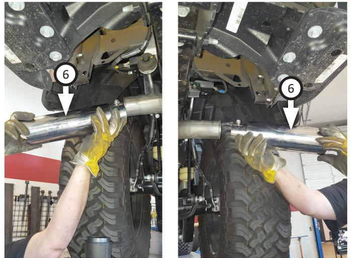
14. Adjust exhaust components for fit; maintaining ½" clearance and compensating for suspension, travel and vibration. Finally, tighten all clamps.
