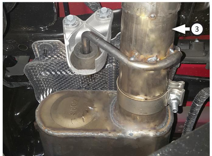
10. Just behind passenger rear tire, unbolt wiring harness bracket. Retain bolts (x2) for later use. Place **clamp (8)** onto **right exit pipe (4)** and connect it to y-pipe right outlet but do not tighten clamp.
