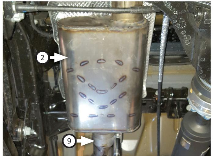
9. Route **y-pipe (3)** over rear axle and connect it to muffler, simultaneously inserting wire hanger into isolator. Tighten clamp just enough to allow for later adjustment.
