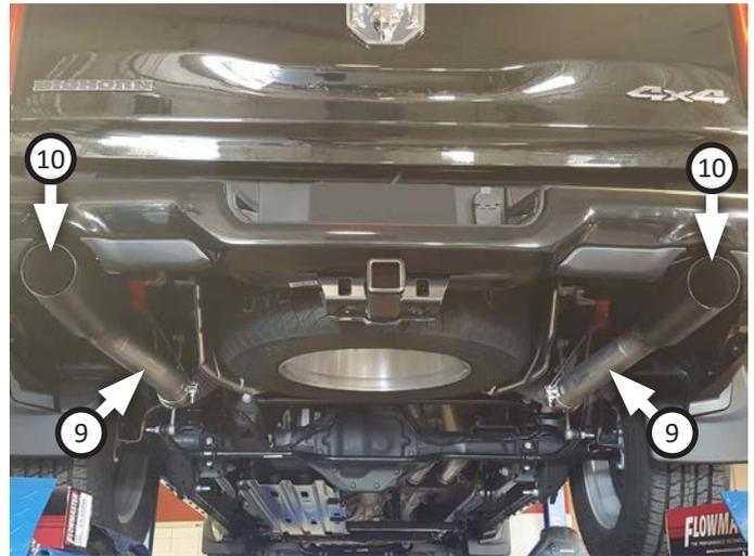
17. Adjust exhaust components for fit; maintaining 1/2" clearance and compensating for suspension, travel and vibration, then tighten all clamps.
