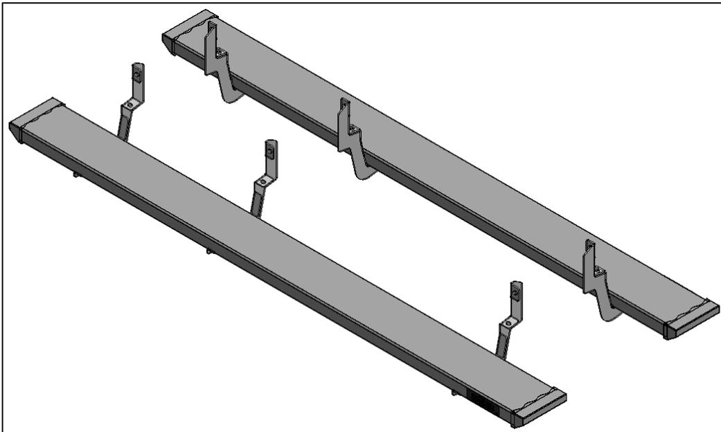
**Step 1:** Beginning with the driver side, remove factory-running bars if equipped and discard. You will see the 8mm threaded mounts in the body. Do the same with passenger side.
