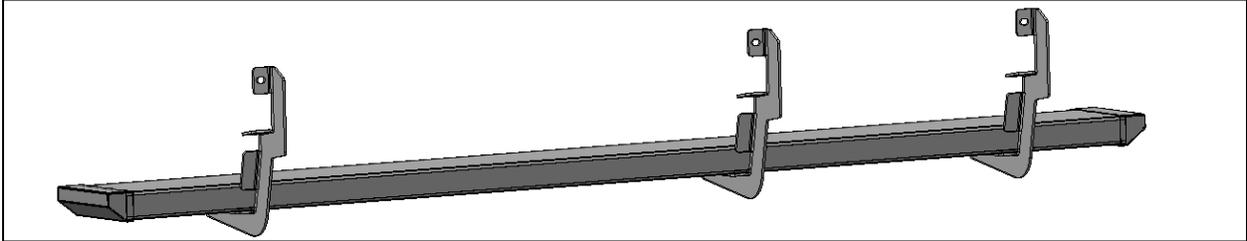
**Step 4:** Insert the supplied threaded brackets (x3) inside the running board lip over the top of each bracket.
