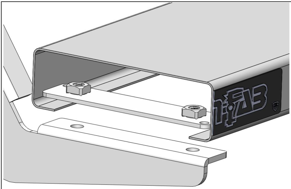
**Step 8:** After final adjustment, tighten all running board threaded mounts.
