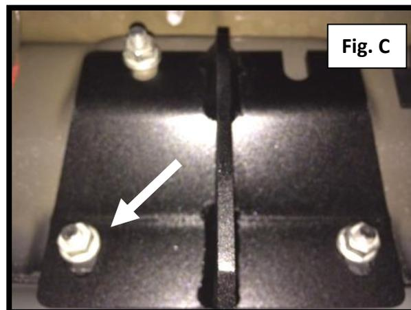
**Step 6:** Move to the front bracket and push tube up leveling with the back and fully tighten all three mounts. Next, fully tighten center bracket and then finish with the remaining mounts on the rear bracket.
