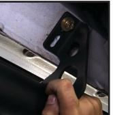
Begin tightening bolts in a alternating pattern. **Avoid using power** or air tools.
