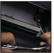
Tighten to 20ft lbs torque to secure the board to the truck. Repeat the same procedure to the other side.
