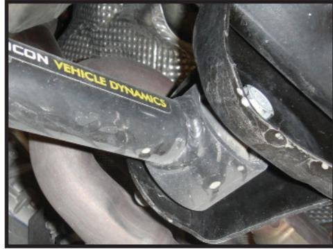
5. Fasten the brake line bracket to the link using the factory hardware. [Torque to factory spec] [FIGURE 4]
