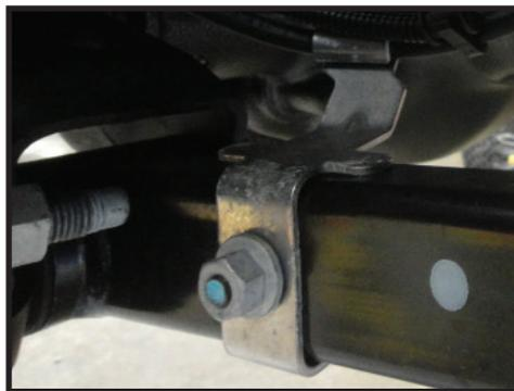
3. Remove the factory front lower link from one side of the vehicle using a 21mm and a 24mm.
