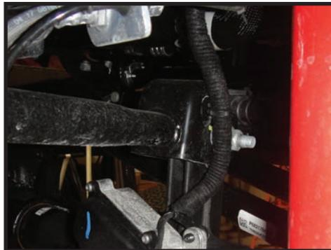
3. Remove the heat shields from the frame mounts using a 10mm socket/wrench.
