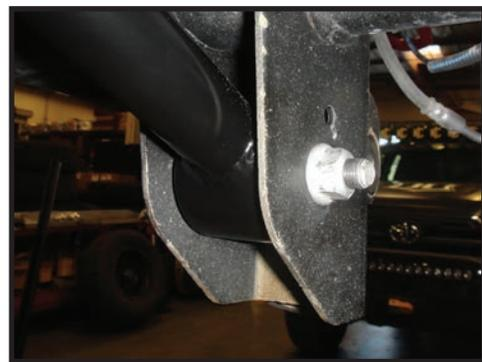
5. Once installed, torque jam nut to 300 ft-lbs.
