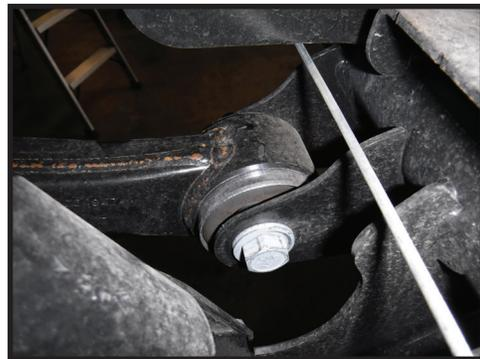
**3.** Mount the rod end to the frame using factory hardware. Pinch bolts should be facing out. Mount the bushing side of the link to the differential using factory hardware. Torque bolts to factory spec using a 21mm and 24mm. [FIGURE 3 & 4]
