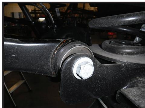
3. Mount the rod end to the differential using factory hardware. Torque bolts to factory spec using a 21mm and 24mm. [FIGURE 3 & 4]
