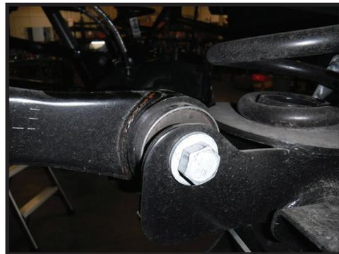
**3.** Mount the rod end to the differential using factory hardware. Pinch bolts should be facing out. Mount the bushing side of the link to the frame using factory hardware. Torque bolts to factory spec using a 21mm and 24mm. [FIGURE 3 & 4]
