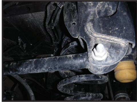
**4.** Torque bolts to factory spec using 21mm.
