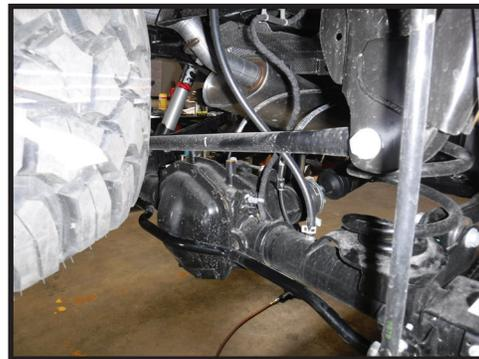
**3.** Install the new track bar with the rod end toward the axle. The pinch bolts should be on top and facing toward the rear of the vehicle. [FIGURE 3 & 4]
