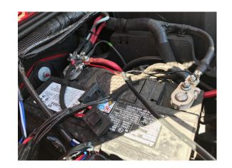
11) Find a secure place to mount the control module. One of our favorite places to mount it is on the subframe next to the battery. Zip tie and tuck away excess wire.
