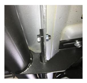
**Step 6.** Adjust the nerf-step where the main bar is level with the body of the vehicle.
