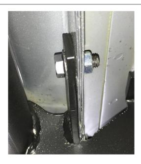
**Step 8.** Next, tighten the remaining hardware that attaches the bracket to the upper body mount.
