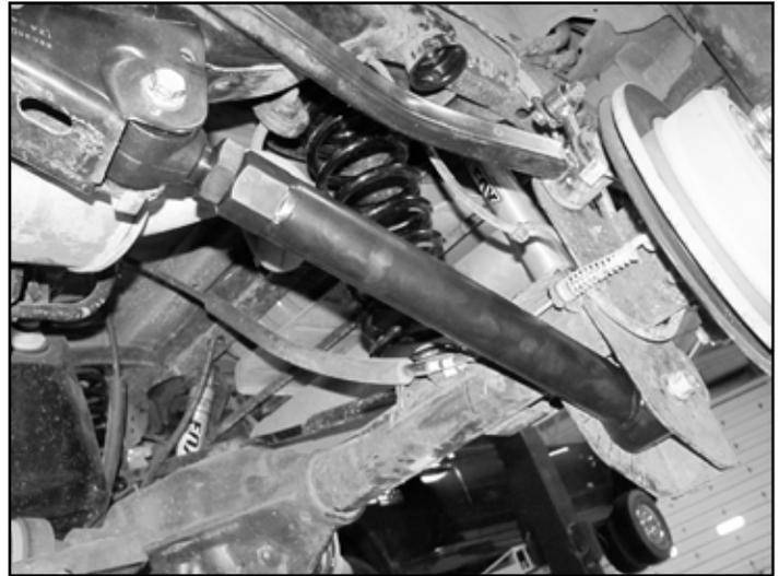
**HINT:** If mounting bolt is difficult to install due to misalignment of Control Arm bushing with mounting bracket, either (1) adjust height of axle housing with hydraulic jack, (2) move axle housing into position with a heavy-duty ratchet strap, or (3) temporarily disconnect track bar until mounting holes align.
