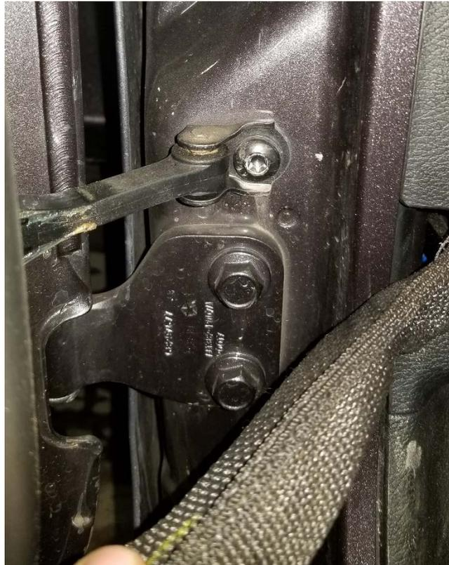
5. With the assistance of a friend, open the door 45° and lift it off of the factory hinges.
