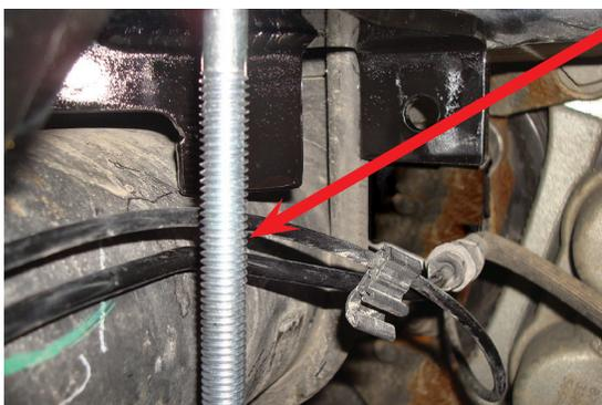
The carriage bolt is always on the outside of the brake line on the passenger's (right) side, regardless of the year.
