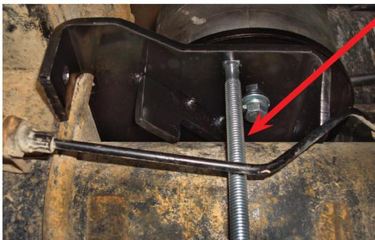
Carriage bolt must be between the hard brake line and axle for this model that has the brake line routed off the axle.
