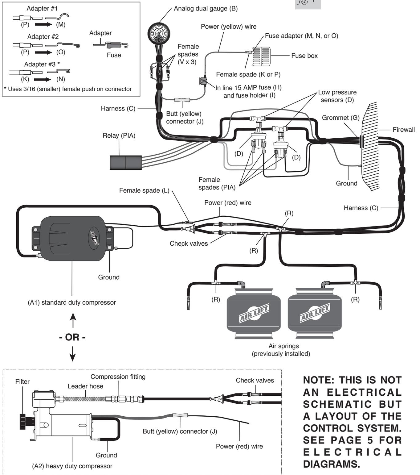
**NOTE: THIS IS NOT AN ELECTRICAL SCHEMATIC BUT A LAYOUT OF THE CONTROL SYSTEM. SEE PAGE 5 FOR ELECTRICAL DIAGRAMS.**
