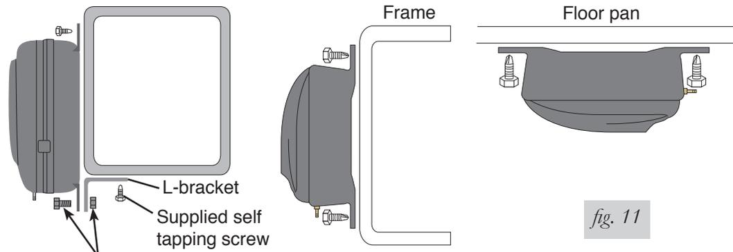
*1/4" Bolt and nut will need to be provided if the L-bracket is fabricated. The L bracket is shown as an optional mounting method and is not supplied.*
