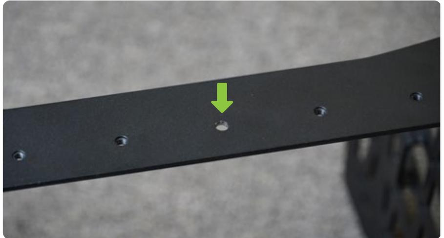
**STEP 2** | Use a 3mm allen head to tighten the bolt while holding the pem nut until it “catches” in the bridge and is secure.
