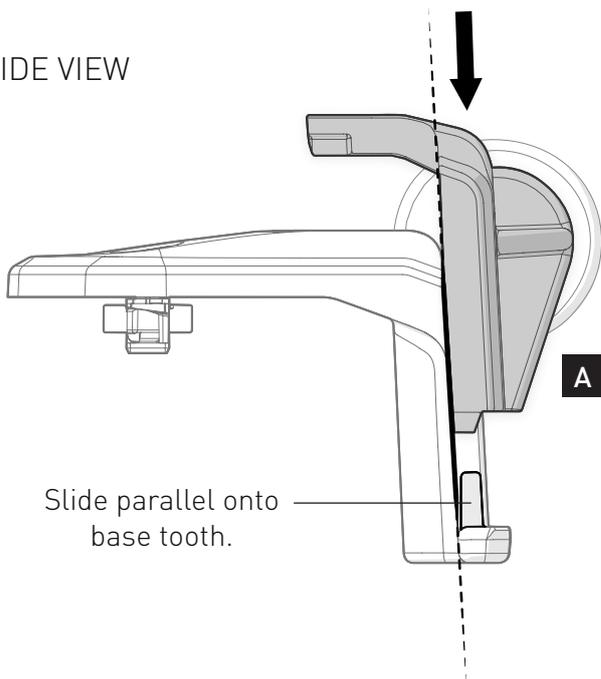
**NOTE:** Ensure adapter catches onto both prongs
