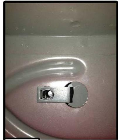
**Step 4.** Align the steps with the mounting holes. Beginning with the middle bracket, use one M8-1.25 bolt and one fender washer for each mounting location and thread the bolts into the mounting holes and leave loose. Continue with the front and rear bracket. **NOTE: Some vehicles require the use of an additional nut and washer for the lower portion of the mounting bracket.**
