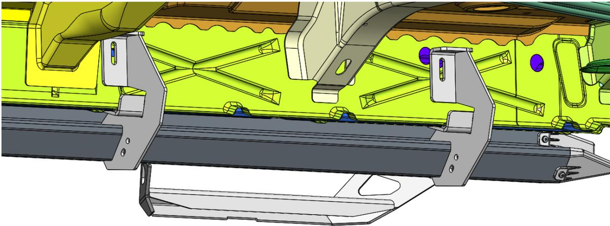
**Step 5.** After final positioning, begin at the rear bracket and tighten the lower bolt to 15-20 ft. /lb. Continue to the front bracket and then to the center bracket. Next, tighten the upper mounts from front to back at 15-20 ft. /lb.
