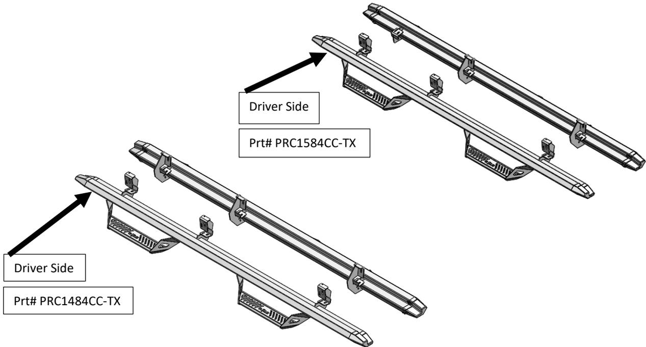
**Step 2.** With the correct step placed on each side of the vehicle, take note of where the brackets are located. Look under the vehicle and locate the factory supplied mounting positions. **NOTE: Some vehicles require the use of supplied clips and nuts.**
