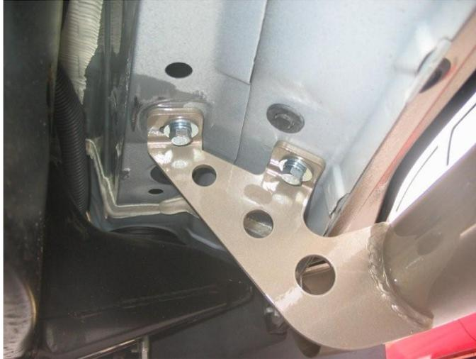
**Step 4** After final adjustment, torque each bolt to 17 ft/lb – 20 ft/lb.
