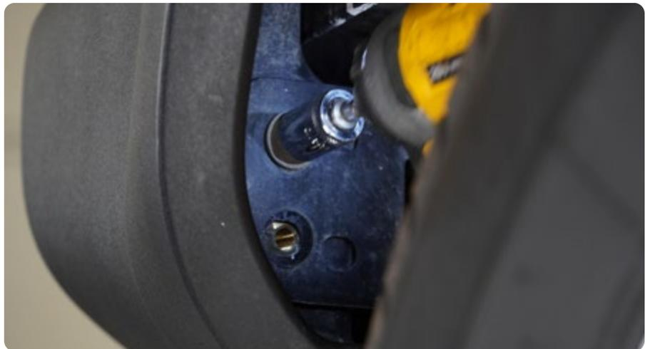
**STEP 5** | Use a 16mm socket to remove the remaining four bolts securing the bumper to the vehicle located between the bumper and rearmost body mount.
