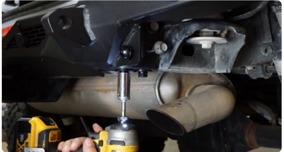
Finish securing all factory hardware using a 18mm or 21mm socket.
