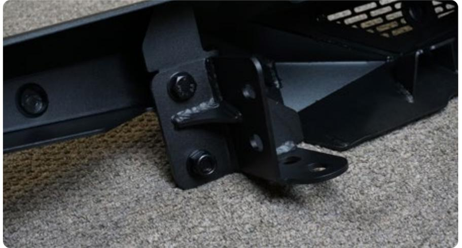
**STEP 11** | Slide the nut plate into the passenger frame rail lining it up with the mounting holes on the bottom.
