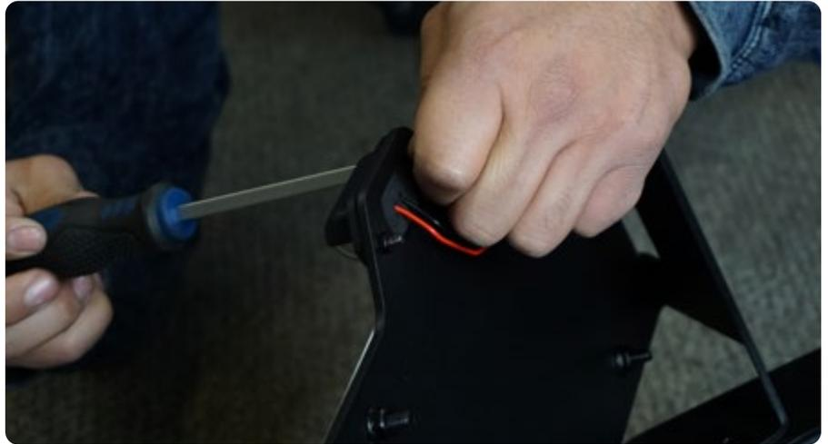
**STEP 9** | If you choose to run pod lights, install these at this time using the hardware provided with the lights.
