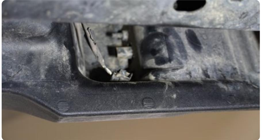
**STEP 2** | Disconnect the bumper wiring harness using a panel clip tool or flat screwdriver to pry open the white locking clip and remove.
