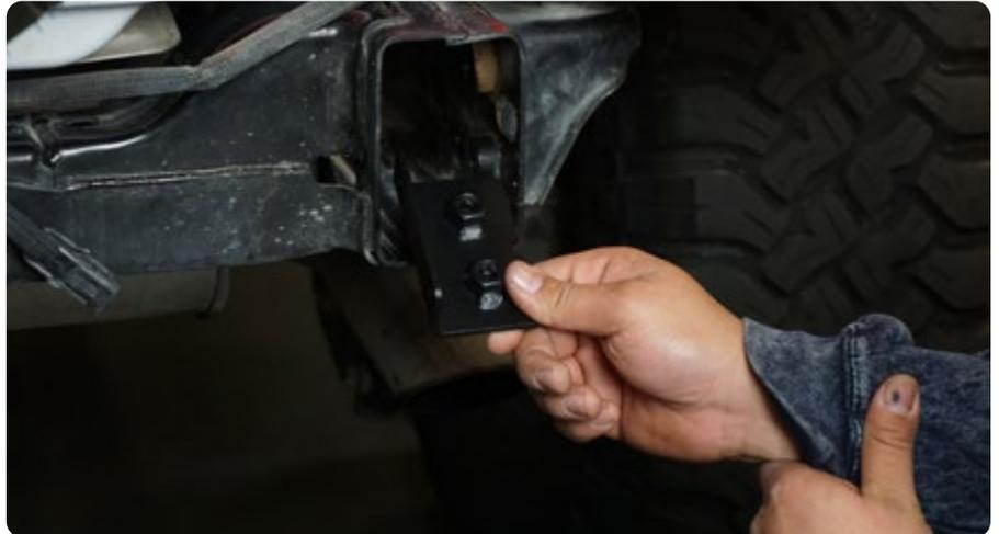
**STEP 12** | Lift the bumper to the vehicle and loosely secure using the factory hardware and a 21mm or 18mm socket.
