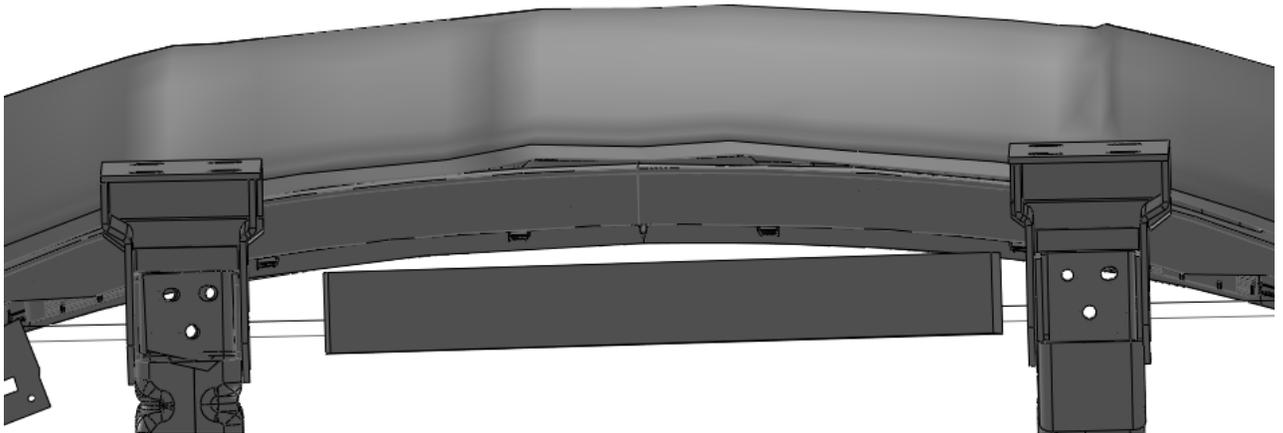
Figure 7 - Intermediate Bracket Orientation (VIEW FROM BELOW)
