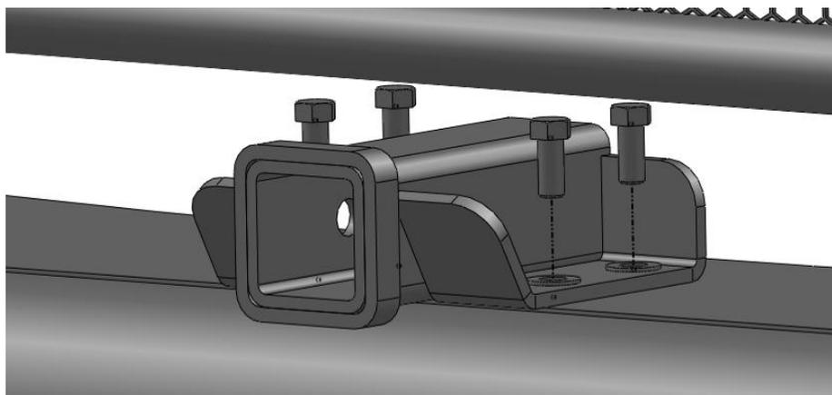
Figure 6 - Hitch Installation
