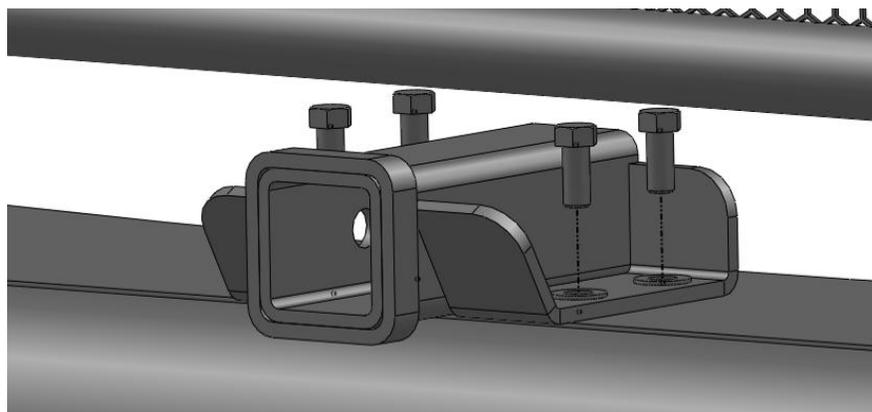
Figure 10 - Hitch Installation
