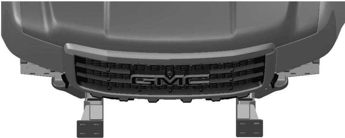
**Figure 11 - Intermediate Bracket Orientation**
