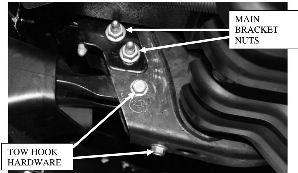
Figure 5 - Tow Hook and Main Bracket Hardware
