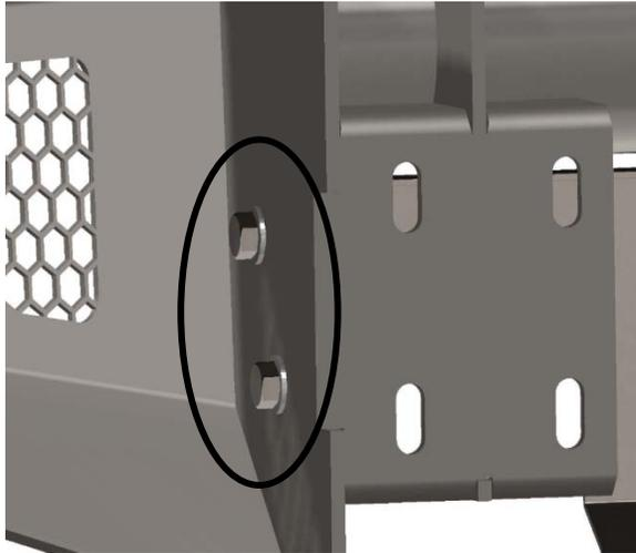
Figure 10a (bolt location for lower guard)
