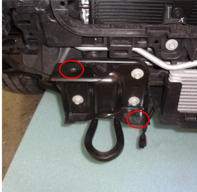
Figure 3a (TOW HOOK & OEM MOUNTING BRACKET)
