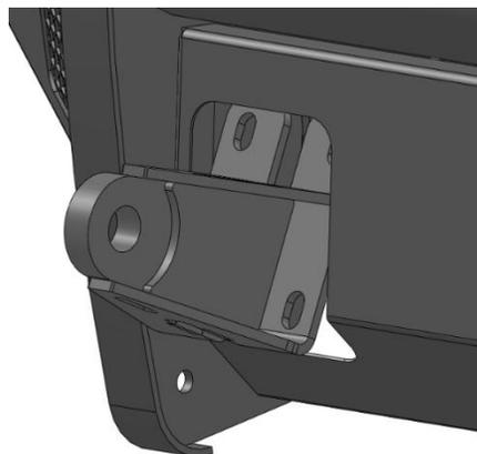
4. **OPTIONAL:** If installing the 2" receiver hitch accessory, attach it to the bumper with the provided 1/2" hardware
