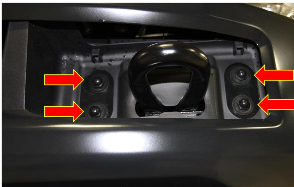
2. Next with the help of someone holding the bumper in place, remove the four 15mm bolts from the bumper support on both sides of vehicle.
