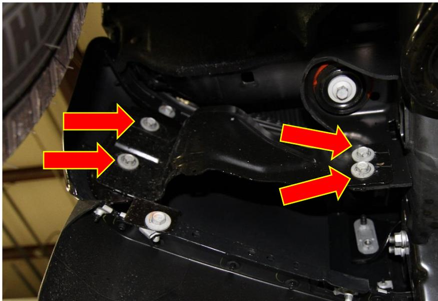
3. The bumper is now ready for removal. (Be careful when removing bumper if vehicle has a block heater as this will have to be unplugged during this step.)
