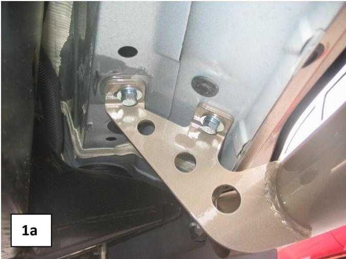
2. Starting with one of the center brackets, start the 8mm hex bolt, 8mm lock washer and 8mm flat washer into the factory bolt locations and hand tighten. See figure 3b. Start all of the remaining 8mm hex bolts, 8mm lock washers and 8mm flat washers. Torque each bolt location to 15ft/lbs.
