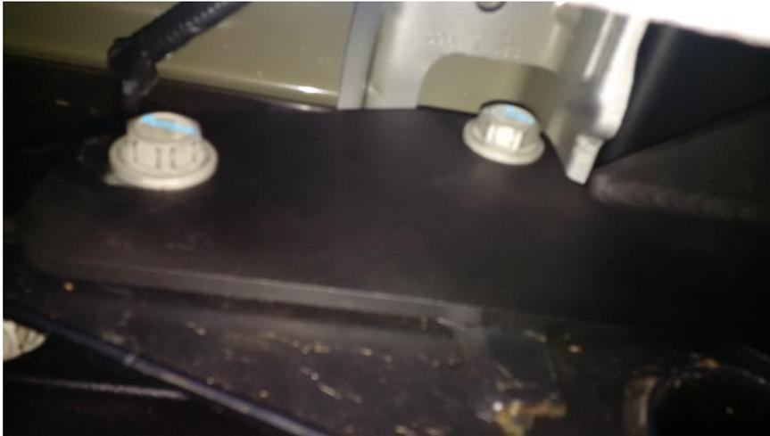
2. Replace the OEM bumper with the Fab Fours Premium Plate Bumper. Use the supplied 1/2" hardware and 3/4" wrench and sockets to fasten the bumper to the intermediate brackets. Do not fully tighten.
