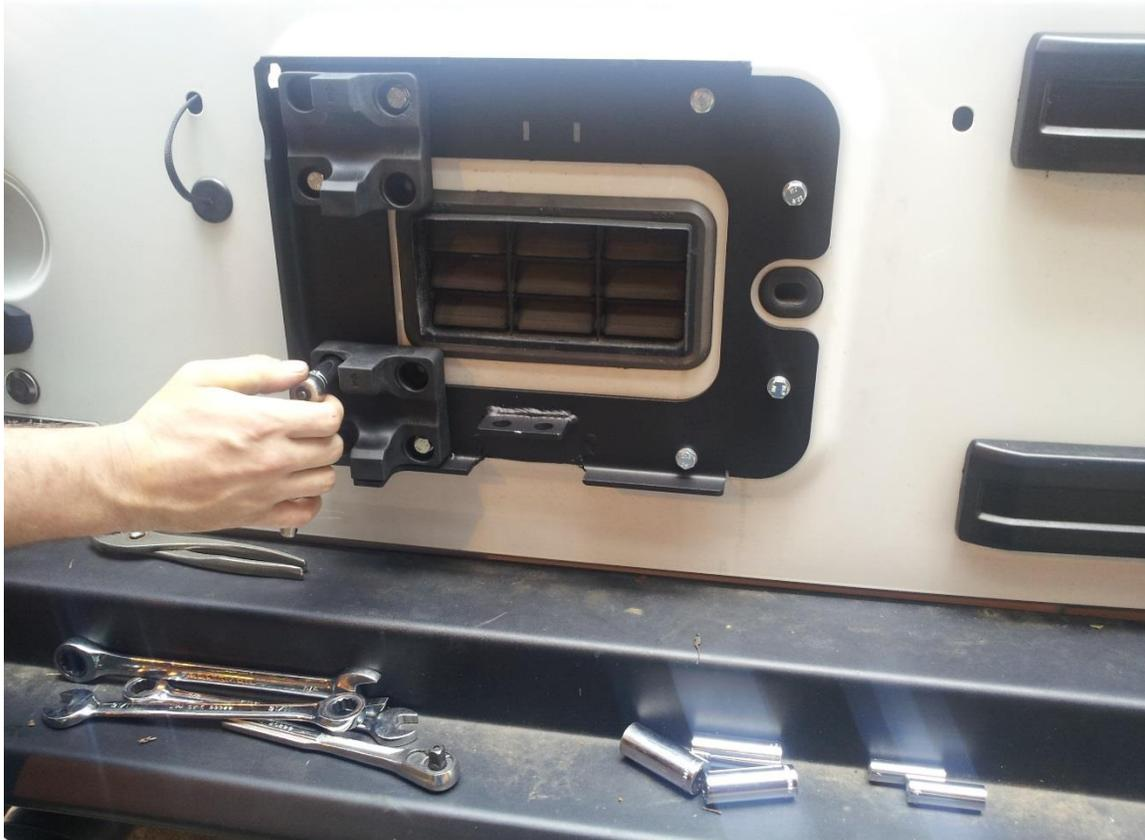
**B. Install pivot shaft using a 9/16" socket or wrench and the provided 3/8" bolt and washer. Do NOT over tighten or use an impact.**
