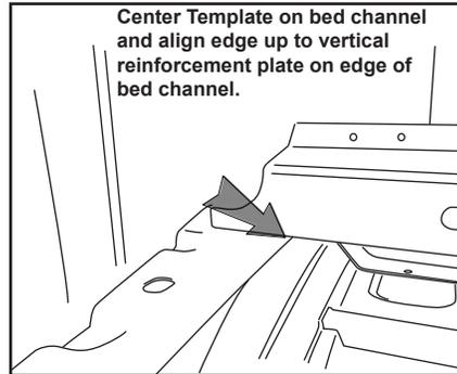
Center Template on bed channel and align edge up to vertical reinforcement plate on edge of bed channel.
