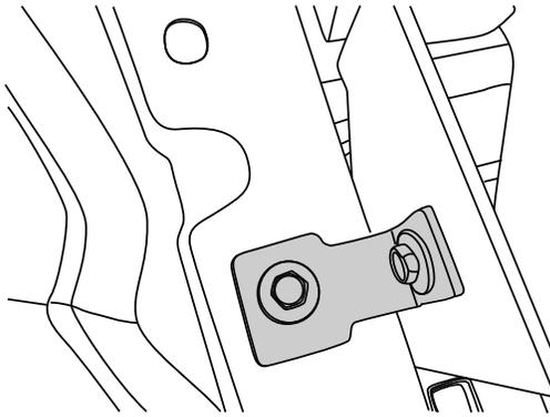
**7** Note: On Rambox models this hole is not present. Mark hole location and drill with a 21/64" drill bit.
