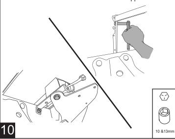
Using "Bracket E" and provided flange head bolt re attach brake cable bracket. Do not tighten.
