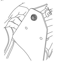
Install Bracket G onto Bracket F and use provided bolts, washer and nut to attach bracket to Front support rib.
