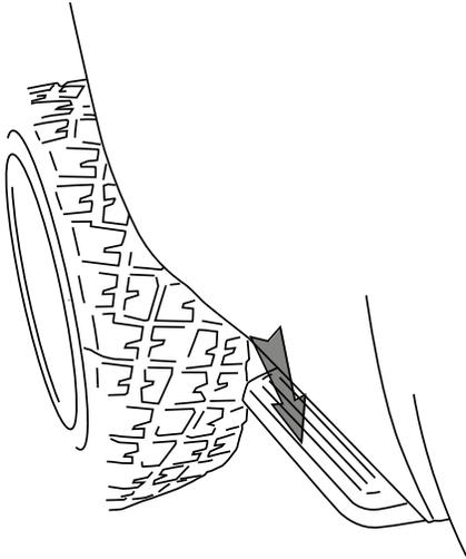
To retract, gently kick up on the underside of the step pad.
