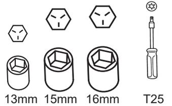
Using a 16mm Socket with extension remove the two body mount nuts and the bumper bracket bolt. **NOTE: Bolt may not be present if aftermarket bumper is on vehicle.**
