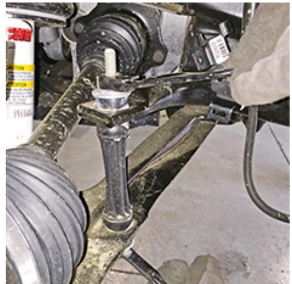
[Illustration 3] Remove the bolts securing the sway bar to the frame and remove the bar. {10mm}
