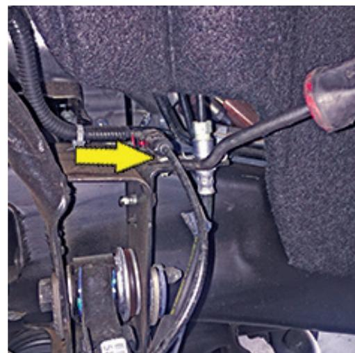
☐☐ [Illustration 7] Locate the brake line bracket on the steering knuckle and remove. {10mm}
