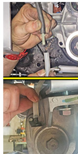
☐ [Illustration 43] Reconnect the differential wiring. Attach the supplied vent hose extension to the factory vent hose and reconnect it to the differential.
