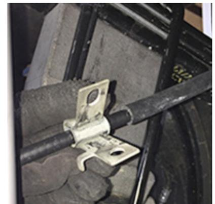
☐ [Illustration 80 & 81] Disconnect the driver side emergency brake cable from brake adjuster at the frame. Collapse the prongs retaining the emergency brake cable in frame bracket and remove. Route the cable over the axle tube, then re-attach it to the frame mount and the adjuster. {vise grips, screwdriver}
