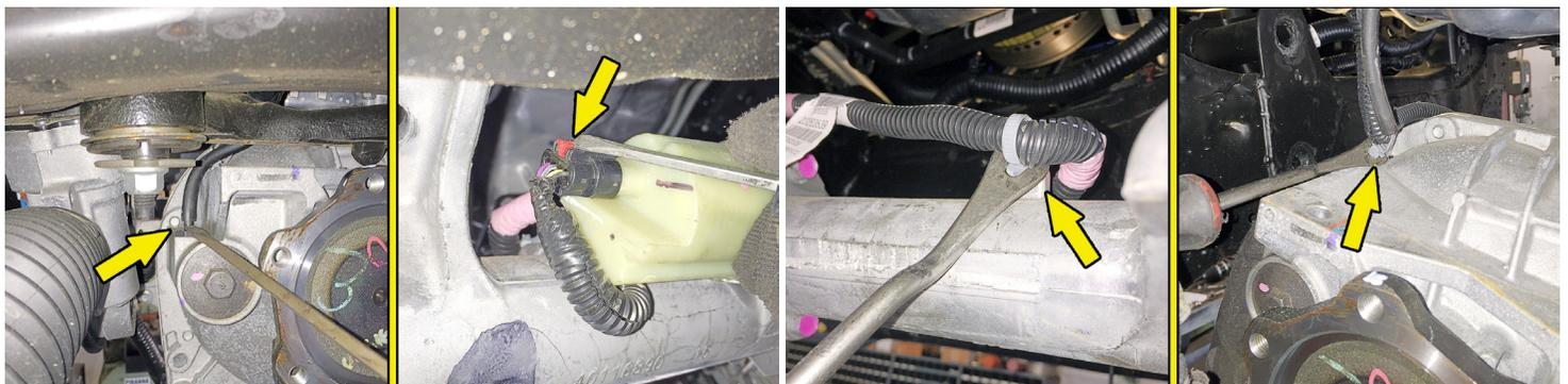
☐ [Illustration 30 & 31] Remove the two differential mounting bolts on the driver side, followed by the two nuts on the passenger side. Carefully lower the differential housing to the floor. {driver side 18mm, passenger side 21mm}
