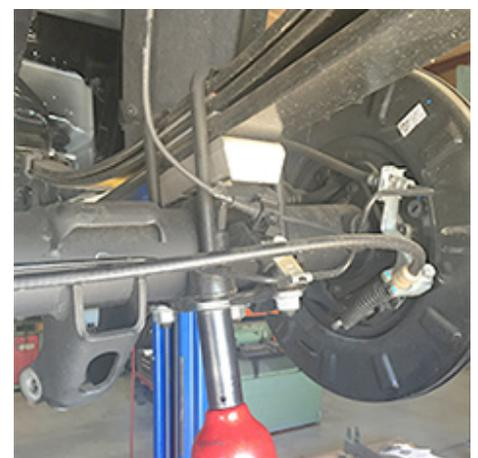
☐☐ [Illustration 91] Clean spring pads of all debris. Position the Superlift block (55-02-201) on top of the axle pad with the tall end facing rearward, then using the floor jack(s), mate the springs to the blocks, be sure that the center bolt heads seat properly. Install the new Superlift 9/16" ubolts (10542) and factory ubolt plate. Evenly torque the ubolts using an "X" tightening sequence. (150) {7/8"}
