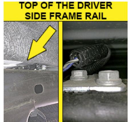
☐ [Illustration 86] Carefully reform the metal lines so that the mounting foot for the bracket lines up with the bottom of the frame rail, directly below its original attachment point. **⚠ CAUTION:** Use extreme caution to avoid pinching or otherwise damaging the lines.
